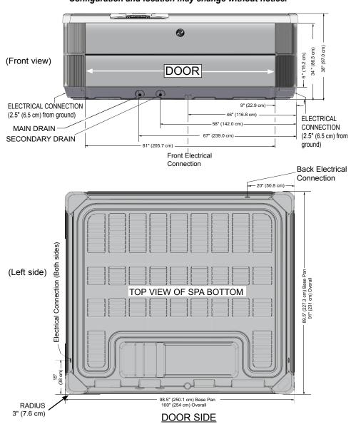
**NOTE: WATKINS WELLNESS** requires that the **ENVOY** be installed on a minimum 4" (10 cm) thick reinforced concrete pad or a deck that is able to withstand more than 120 lbs/ft² (570 kg/m²).
