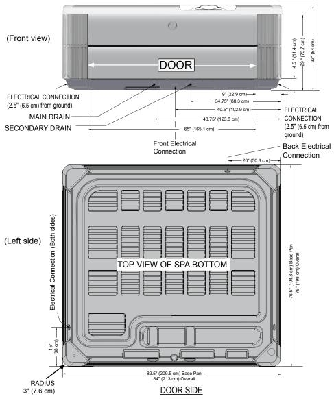
**NOTE: WATKINS WELLNESS** recommends that the **PRODIGY** be installed on a minimum 4" (10 cm) thick reinforced concrete pad or a deck that is able to withstand more than 125 lbs/ft<sup>2</sup> (595 kg/m<sup>2</sup>).
