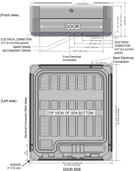
**NOTE: WATKINS WELLNESS** recommends that the **SOVEREIGN** be installed on a minimum 4" (10 cm) thick reinforced concrete pad or a deck that is able to withstand more than 115 lbs/ft² (555 kg/m²).
