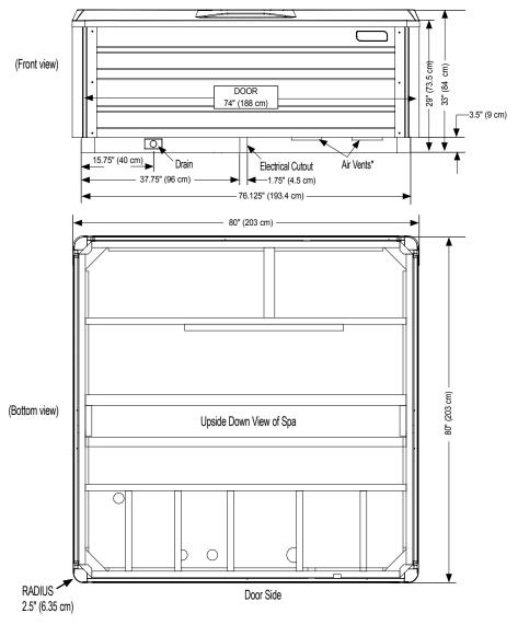
NOTE: WATKINS WELLNESS recommends that the BEAM be installed on a minimum 4" (10 cm) thick reinforced concrete pad or structurally sound deck able to support the "dead weight" found in the spa specification chart. WARNING: The BEAM must not be shimmed in any manner.
