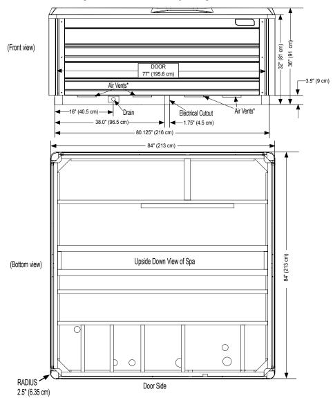
**NOTE: WATKINS WELLNESS** recommends that the **FLASH** be installed on a minimum 4" (10 cm) thick reinforced concrete pad or structurally sound deck able to support the "dead weight" found in the spa specification chart.
